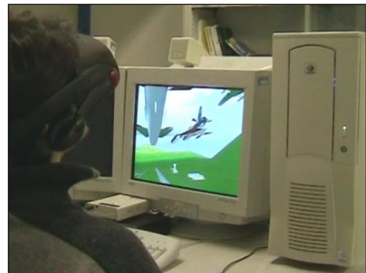
Figure 3. Guided navigation mode. User position is constrained (e.g. inside an aircraft); Viewpoint orientation changes following user’s head (3DOF sensor mounted on HMD).
