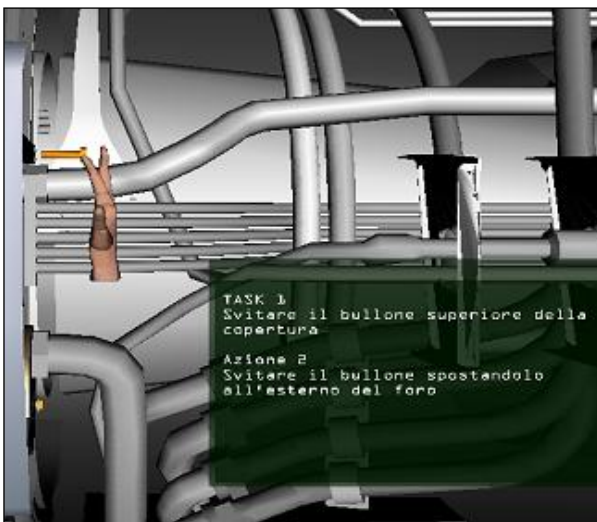
Figure 8. Unscrew the bolt (using “finger-screwdriver”).
