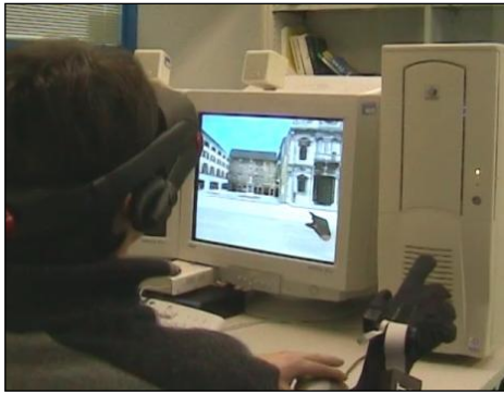
Figure 4. Free navigation mode. Body position, velocity and orientation are driven by hand gestures; viewpoint follows user head orientation (as in the real world).
