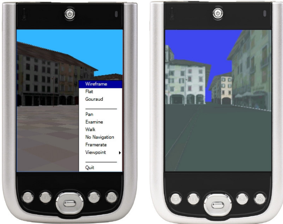
Figure 1. The MobiX3D player [13] displays 3D content (described in the ISO standard X3D) on mobile devices; it can be downloaded from http://hclilab.uniud.it/MobiX3D
