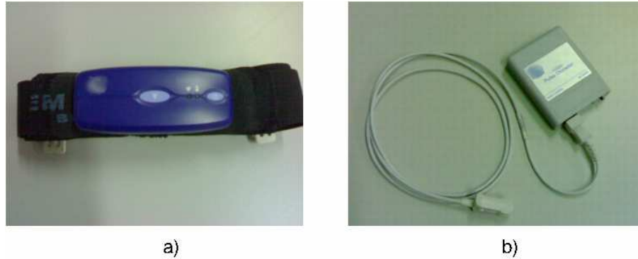
Fig. 2. Sensors currently managed by the Context Analyzer. a) heart rate monitor with integrated 3D accelerometer b) pulse oximeter.
