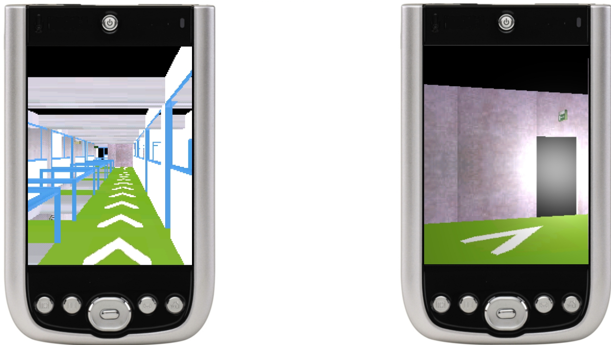
Figure 1: A 3D model augmented with evacuation instructions. Paths are represented by arrows (left figure), while landmarks are highlighted by spotlights (right figure).
