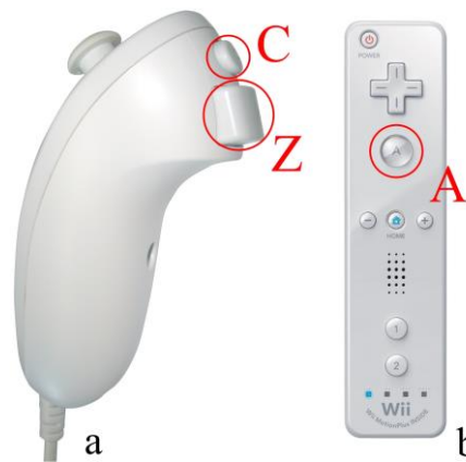
Figure 4. The Nintendo Nunchuck controller (a) and the Nintendo Wii Remote (b). The C, Z, and A buttons are circled.
