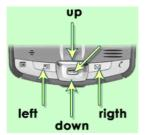
Fig. 2. The hardware buttons used to control the device
